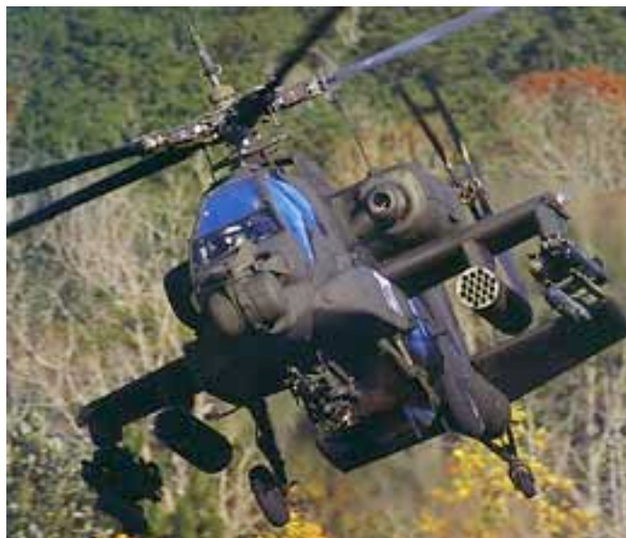
Here you can see the 30mm canon, and the right landing gear is easy to see, while
