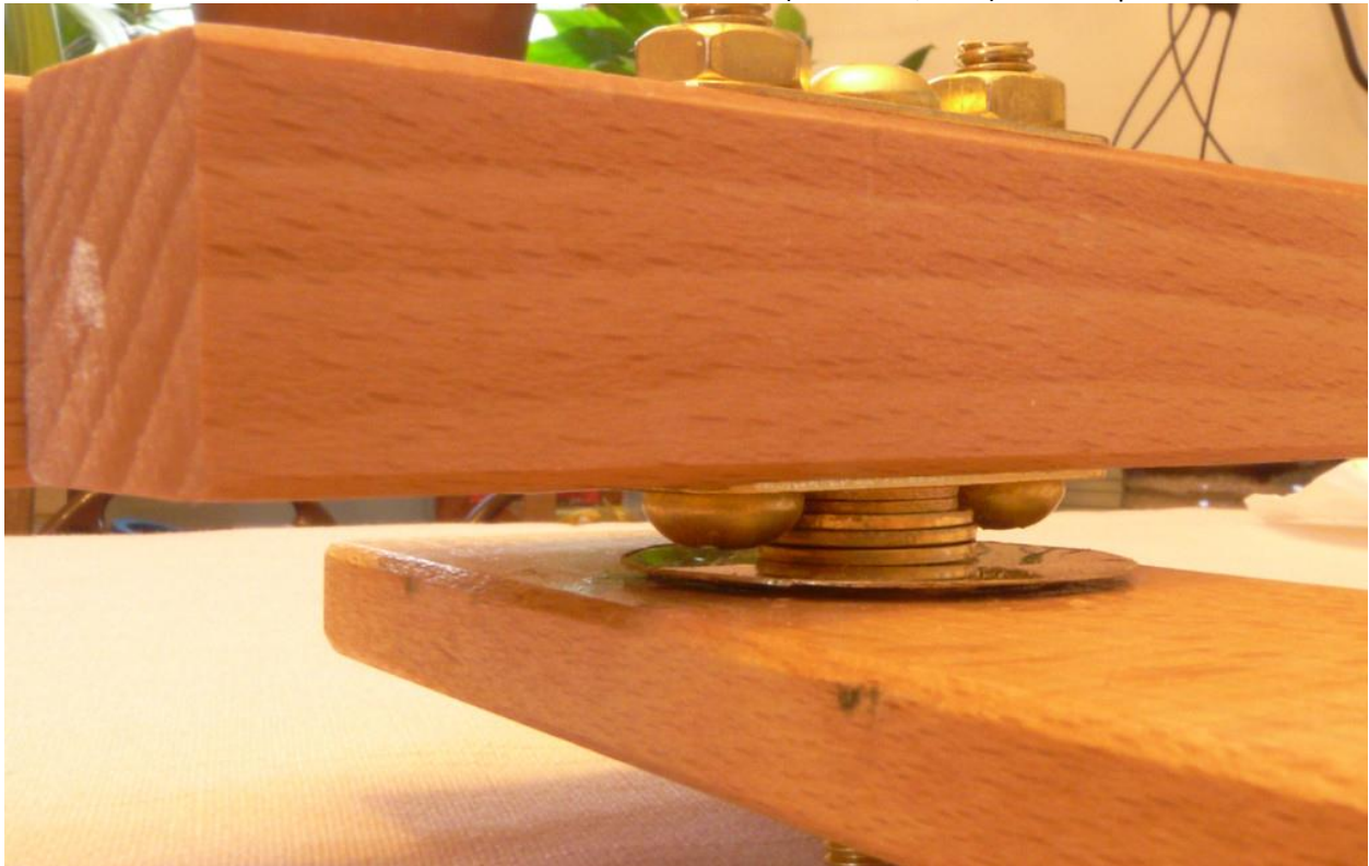
Figure 15 - Preventing marring of the back of the crossbar. Crossbar is at the bottom. Right leg is the square bit of wood on top. Several brass washers have been added to the pivot screw for the crossbar, plus a large thin washer. These ensure that the crossbar can't rub on the two screw heads you see at the left and right of the stack of washers.
