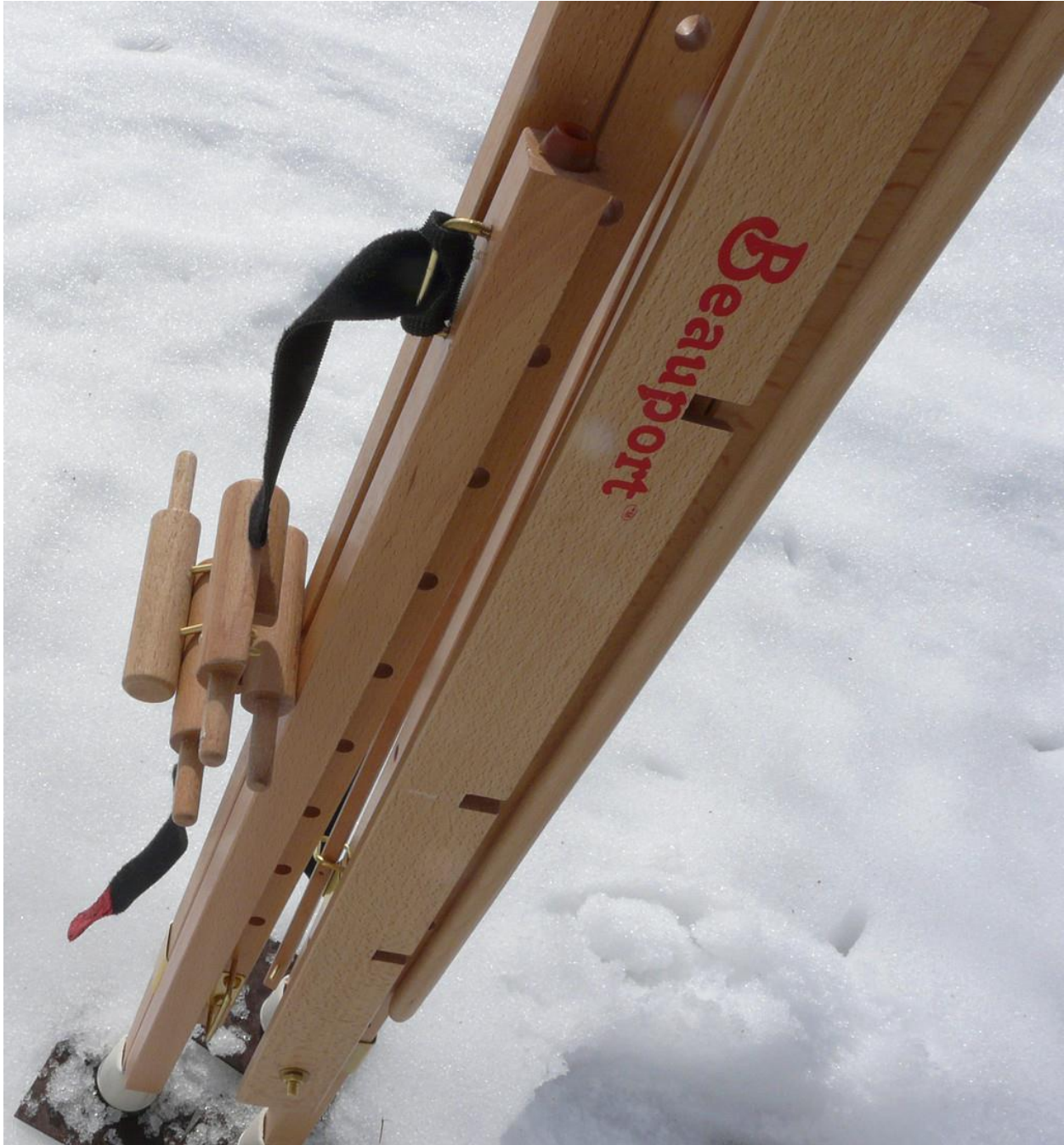
Figure 14 - Better view of combo strap on leg extension. Strap is affixed to the added brass staple, the leg swung upside down, and the extension's three pegs merely stuck into the corresponding three holes on the left leg.
