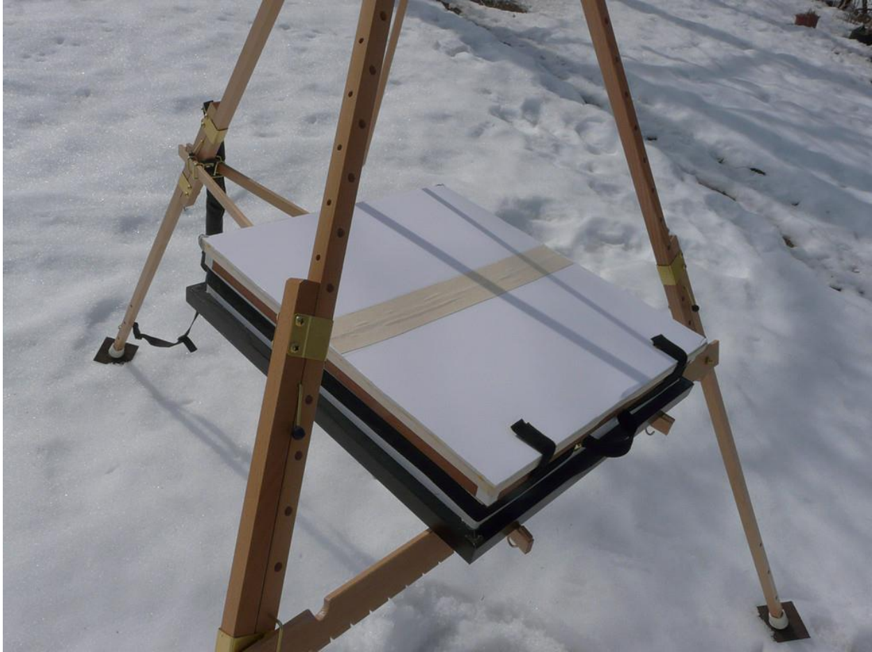
Figure 18 - Box on support sticks, closed. Relatively big – 20 x 24 inches or so. The “latches” are simply pieces of a second Velcro strap, one set glued on the box front with fuzzy side out (won’t stick to clothes or coats), one set on the top (also fuzzy side up – the inner-facing hooks on the front closures engage with the fuzzy top bits). Before cutting up into closure chunks, this strap was identical to the one used for the combo strap (Tweak 10). The hinge in center of the lid is a strip of artist’s canvas, gesso side glued down.
