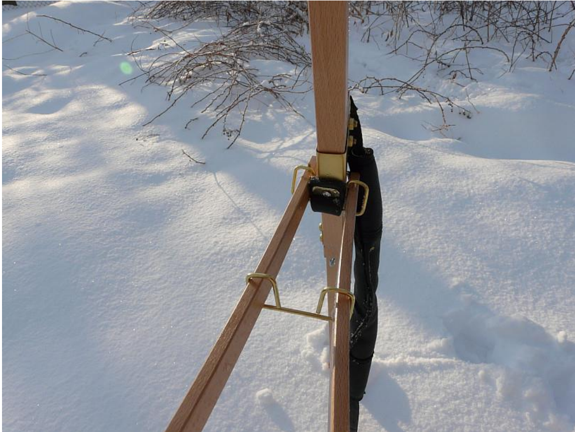
Figure 8 - "Use the metal holder as tension support by sliding forward to ensure the sturdiness of the easel," the Beauport instructions say. Here the C-wire ("metal holder") closest to you has been pulled forward to squeeze the legs to stiffen them. It is difficult to do this effectively the way the easel is shipped.
