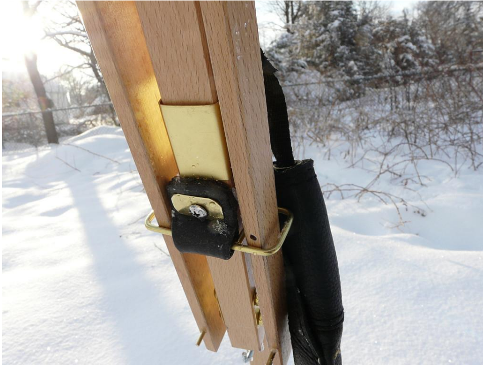
Figure 7 – Heavy leather hinge or mount for permanently affixing the two supporting sticks (the sticks are in the up or parked position). This hinge was made from a $3 thrift-store purse and buttoned down with a hand-cut chunk of brass and a screw. The rectangular brass above the mount isn't part of the hinge. It's the follower or brace that's part of the leg adjusting mechanism.
