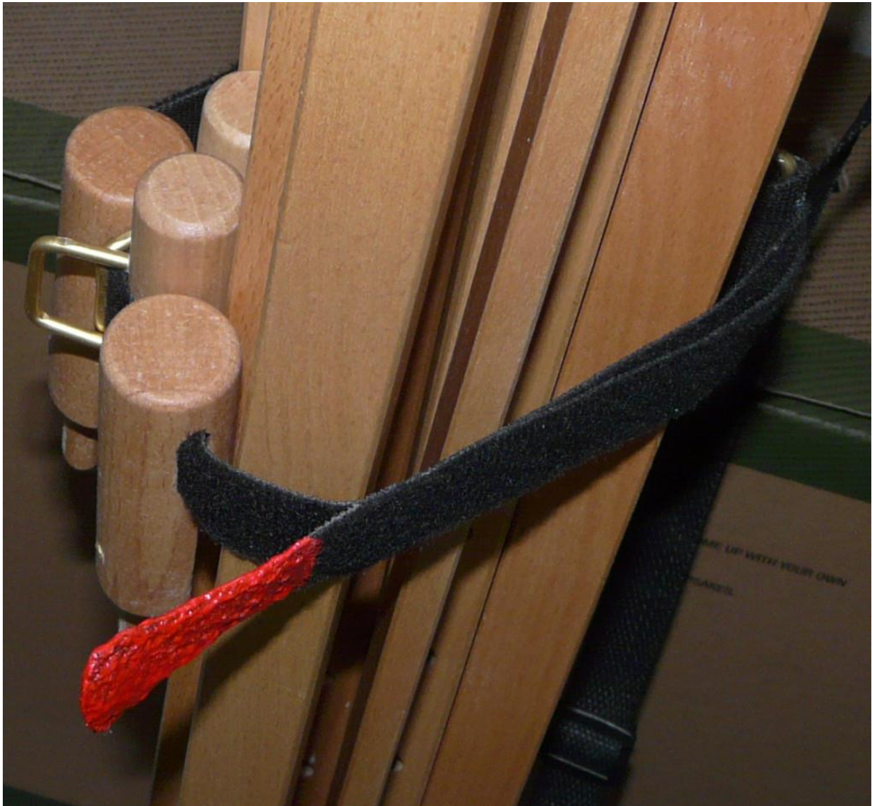
Figure 13 - Combo easel wrap and peg strap. Velcro strap runs from a brass staple added to one of the extension legs (not visible). The strap has a red coating on the near end for visibility and to provide a handy pull tab. The canvas pegs slide onto the strap.
