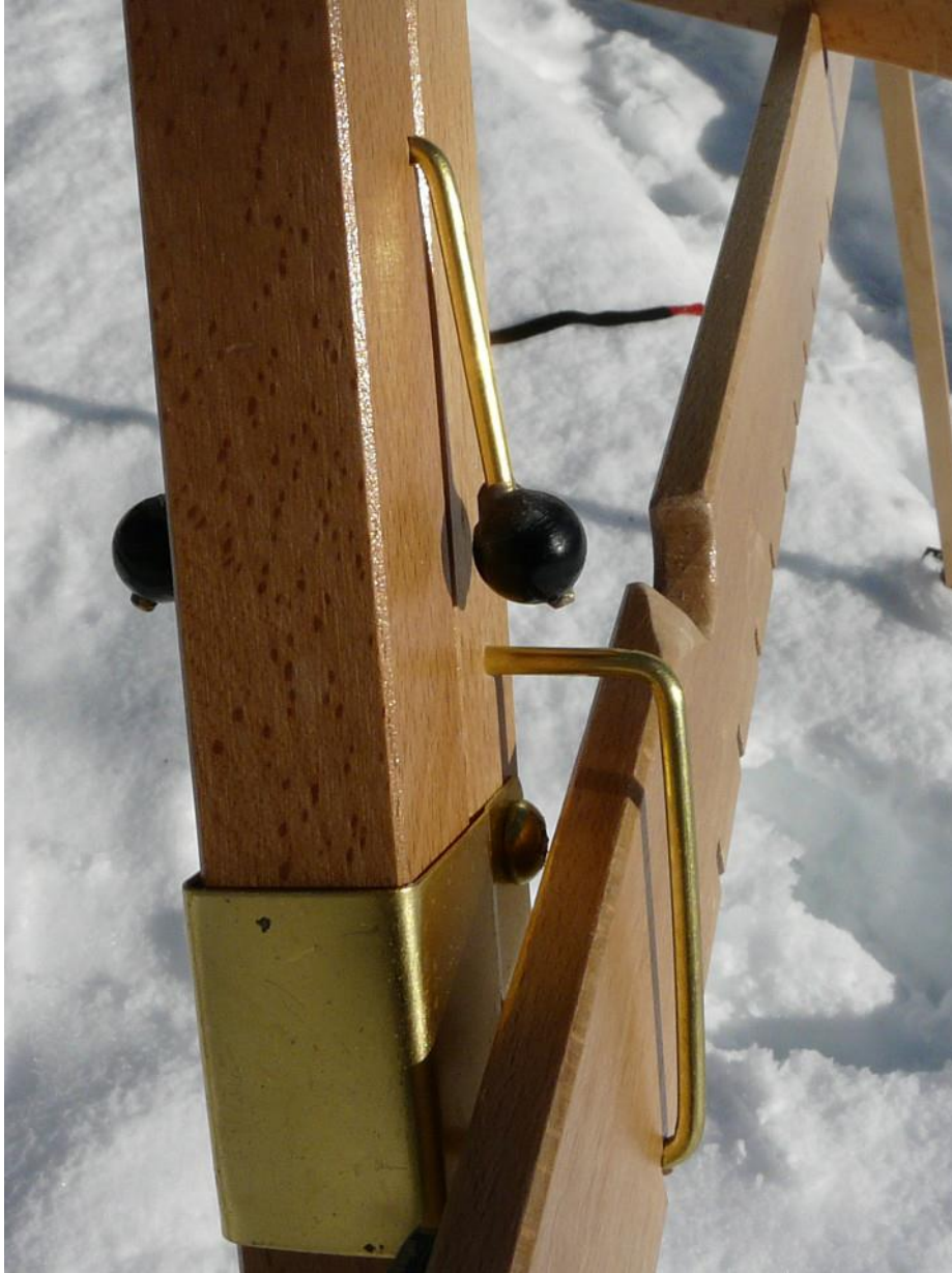
Figure 9 - Knobs epoxied onto the wire adjuster on left leg. The cut-out visible on the crossbar just behind the brass staple on the left leg is part of later madness. It accommodates the parked knobs on the right leg and allows the crossbar to stow fully upright when pivoted up.
