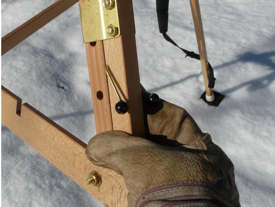
Figure 10 - Knobs allow easy leg length adjustment while wearing heavy gloves. In the summer, the knobs protect your sensitive artist's fingers. Note the showshoe on back leg (Tweak #12, below)
