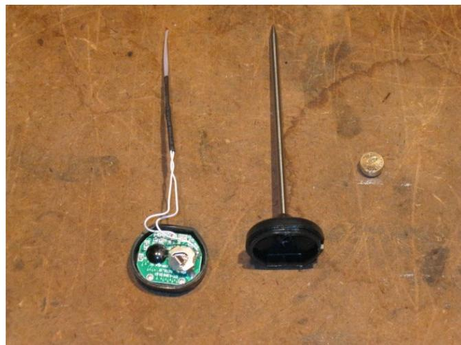
The head is removed by pulling and twisting while the probe housing itself is held firmly in the vise. Lately I have been sticking the removed head in the freezer for a day or so to make the glue removal much easier.
