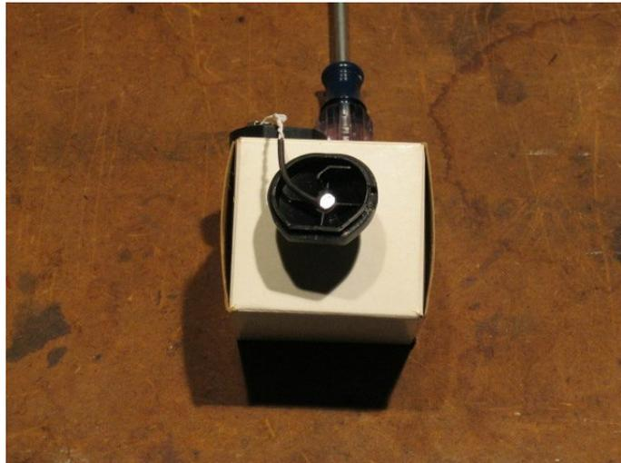
The wiring is wedged between the body and a plastic piece which ensures that the thermistor tip is "bottomed out" in the probe housing.
