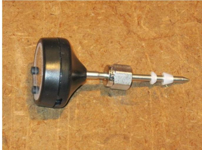
The thermometer inserted into the custom adaptor shown with the plastic thread protector (removed).
