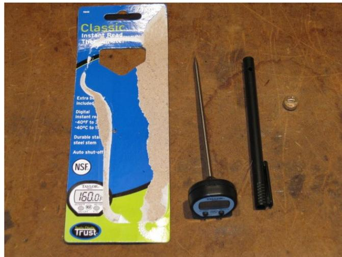
The thermometer itself comes apart with a coin or your fingernail. The “guts” of the thermometer can be a little tricky to remove given the presence of glue used during original build. A hot air gun and steel picks usually will do the job.
