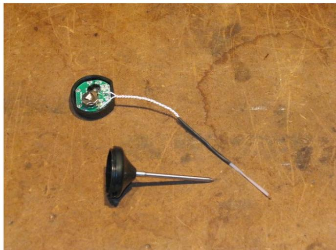
A dab of thermal paste is applied to the thermistor bead to ensure good thermal conductivity between the stainless steel probe housing metal and the thermistor.
