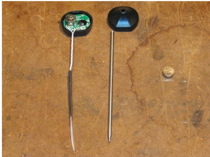
The body of the thermometer is machined for increased internal clearance.
