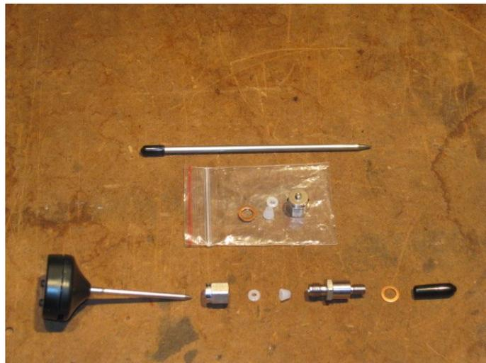
This is a pic of a replacement thermometer "kit" but also a thermometer prior to installation into the adaptor.
