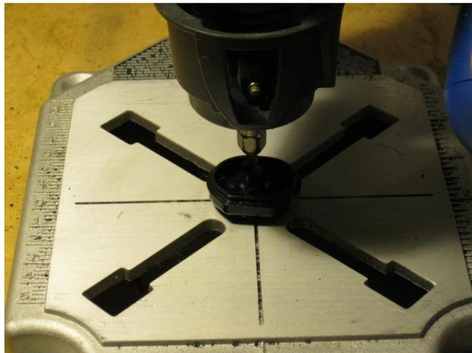
The body is reamed to ensure a tight fit with the custom probe housing.
