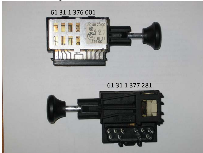
Fig 3: Early (Top) and Late E30 Headlight Switches
