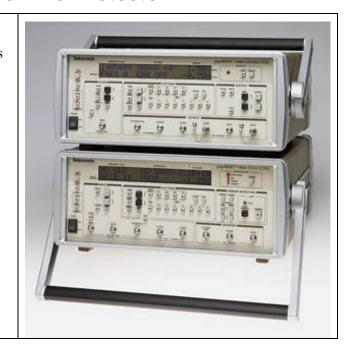
The GB1400 is a general-purpose 1400 Mb/s bit error rate tester (BERT) built to meet the exacting standards of design engineers who need to verify and characterize high-speed serial data transmission circuits, interfaces and systems. While primarily a lab instrument, the GB1400's compact design, full computer programmability and relatively light weight also enable it to serve in manufacturing ATE and field test applications.
